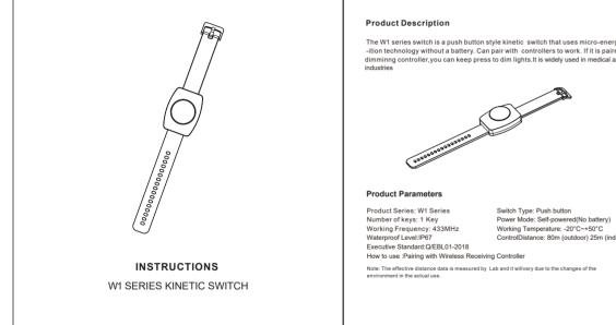
The W1 series switch is a push button style kinetic switch that uses micro-energy acquis -ition technology without a battery. Can pair with controllers to work. If it is paired with a dimminng controller, you can keep press to dim lights. It is widely used in medical and pension
